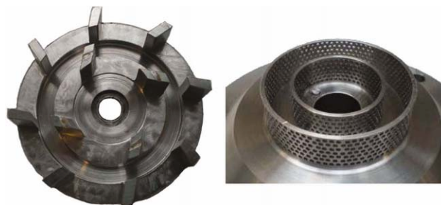
Figure 2. Standard double emulsification screen setup (a) the rotor (b) the screens.
