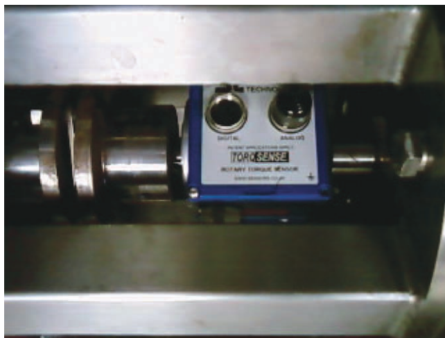
Figure 4. TORQSENSE torque meter fitted to Silverson drive shaft.
